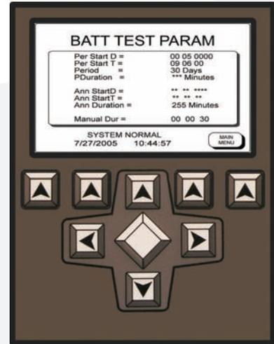
The LCD display on the model “ELE” *Intellistat* provides all electrical parameters, inverter status, programmable inverter and battery testing, remote monitoring and reporting, and data logging. An optional integrated fax modem can be included in the closed-loop communications system.
